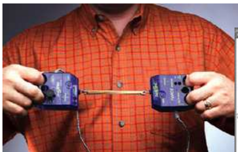
Demonstrating Newton's 3 rd Law with two force sensors
