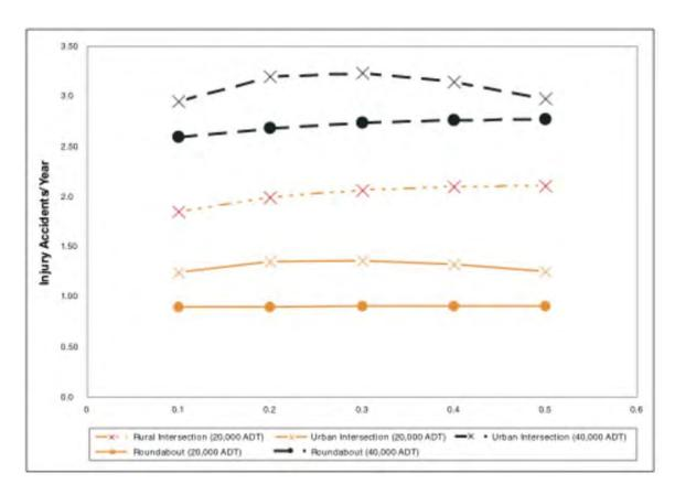
FIGURE 4 - COMPARISON OF PREDICTED INJURY CRASHES FOR SINGLE-LANE AND DOUBLE-LANE ROUNDABOUTS WITH RURAL OR URBAN SIGNALIZED INTERSECTIONS. (Source: FHWA)
