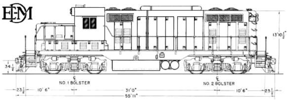
FIGURE 35: DIAGRAM FOR ENGINES 1501 AND 1502
