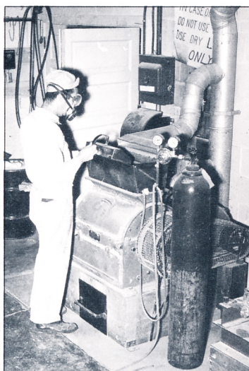
The garbage hog used to cut up calcium and magnesium for the reduction process.
