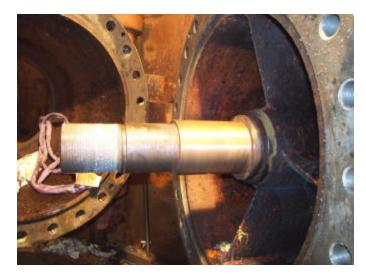
Existing housing and guide vanes. Note: Poor existing surface finishes Figure 6
