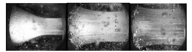
20 % Needle stroke 40 % Needle Stroke 90 % Needle Stroke Actual video stills of single jet in operation Figure 3
