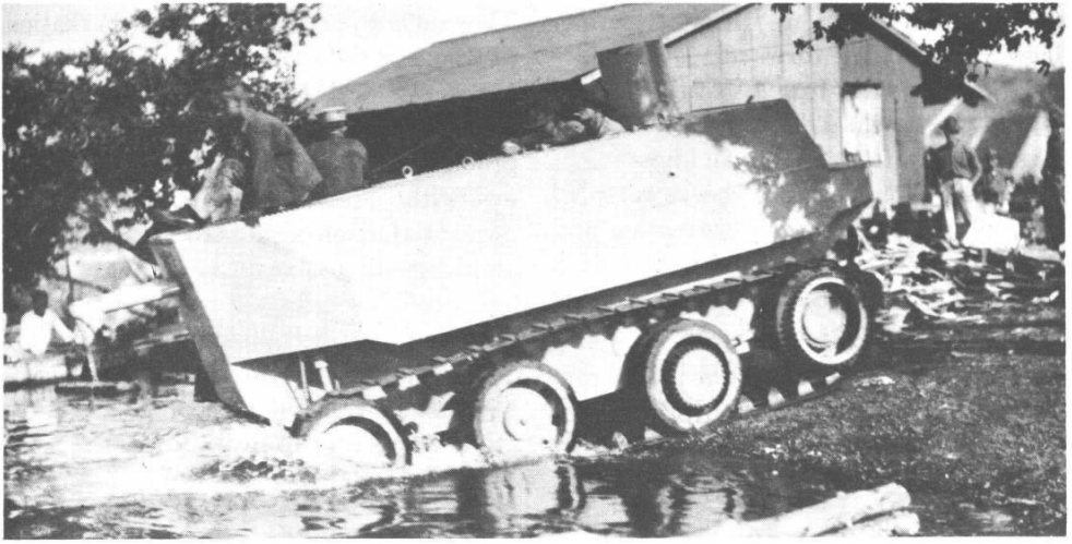
EXPERIMENTAL AMPHIBIAN TRACTOR developed for the Marine Corps in 1924 began the long line of test vehicles that culminated in the LVT. (USMC 13562)
