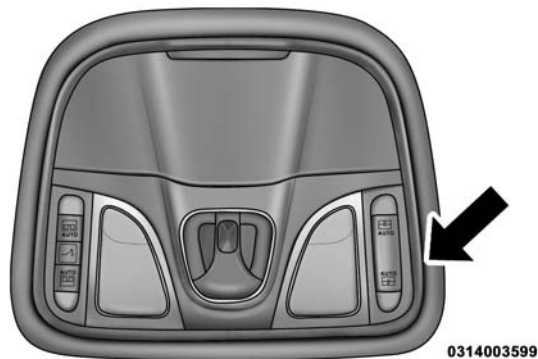
Power Shade Switch
