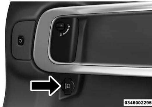
Rear Power Outlet
