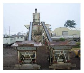
If the exact dimensions of the hopper are not available, the hoppers are generally about 12 feet by 12 feet, and about 10 feet tall. The bottom of the bucket of the front-end loader can be assumed to be 3 feet above the top of the hopper when dumping material. There may be more than one hopper, and the hoppers may be used for different materials (e.g. sand vs. aggregate). Therefore, the emission rate may not be the same for each
