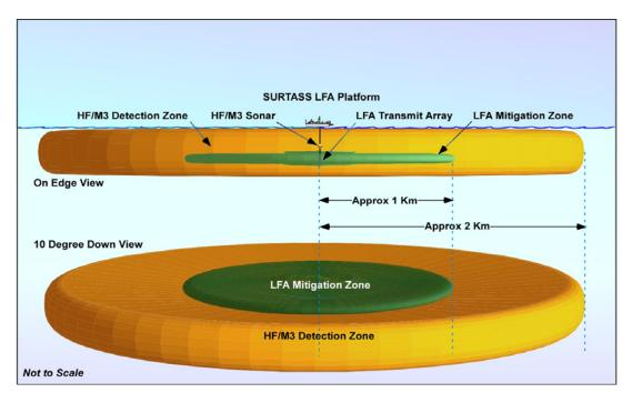
Figure 2. HF/M3 Sonar Detection and LFA Mitigation Zones
