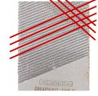
**Double-Cut** files have two sets of diagonal rows. The first set is called the overcut. The second set is cut at a different angle with the file axis, and is known as the upcut (it is finer than the overcut).
