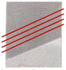
**Single-Cut** files have a single set of diagonal rows of teeth, parallel to one another and extending across the working face of the file.
