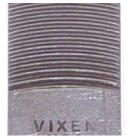
**Curved-Cut** is an arrangement of file teeth in curved contours across the working face of the file. The teeth are milled with a decided undercut (or positive rake).
