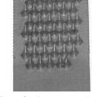
**Rasp-Cut** is a pattern where each tooth is individually formed by a single-point tool or punch - the teeth are formed separately and are disconnected.
