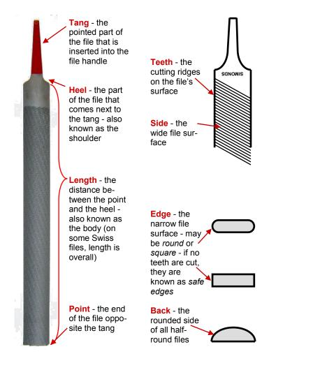
**Cut** - The character of the file teeth. The four standard file cuts are: Single-Cut, Double-Cut, Rasp-Cut and Curved-Cut. Curved-Cut.
