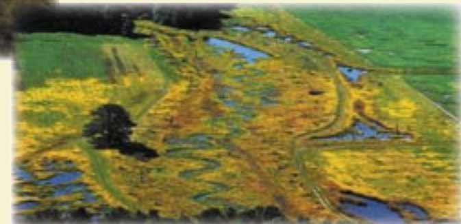
Traditional tax ditch restored to replicate a natural floodplain with sinuous low-flow channel
