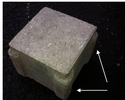
Beveled spacers along the edges of paver blocks create the gaps between each interlocking concrete paver where water can infiltrate.
