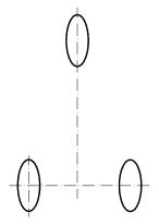
Figure 3. S - Single Wheel Main Gear with Single Wheel Nose Gear
