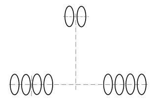
Figure 19. Q - Quadruple Wheel Main Gear with Dual Wheel Nose Gear, Hawker Siddeley HS-121 Trident
