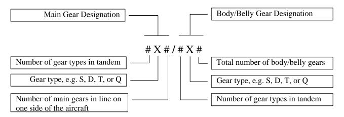
Figure 1. Aircraft Gear Naming Convention
