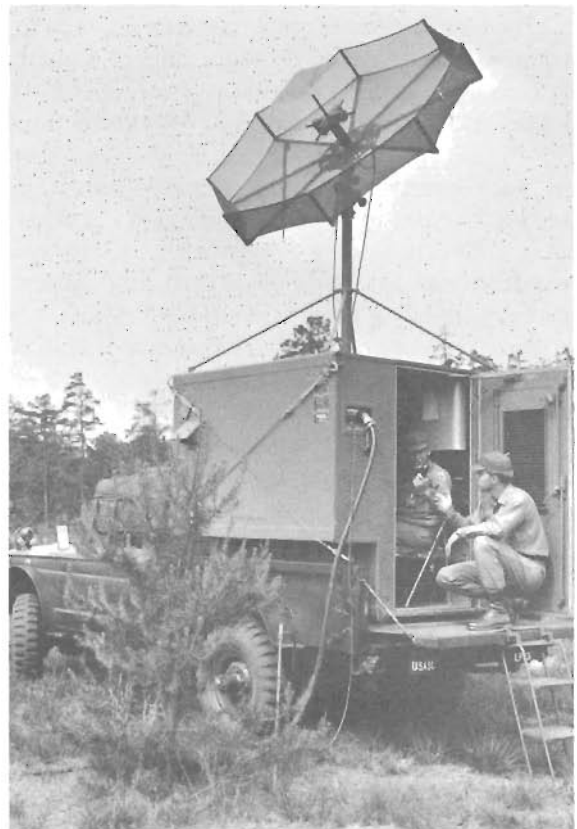
Figure 7. Satellite communications shelter installation AN/TRC-157.
