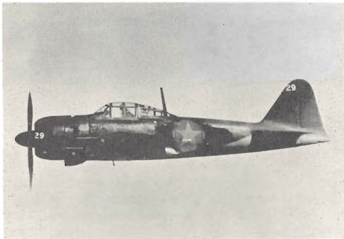
Figure 7. Captured Mitsubishi 00. This is the Navy version (Zeke) of the Army fighter known as the Zero.
