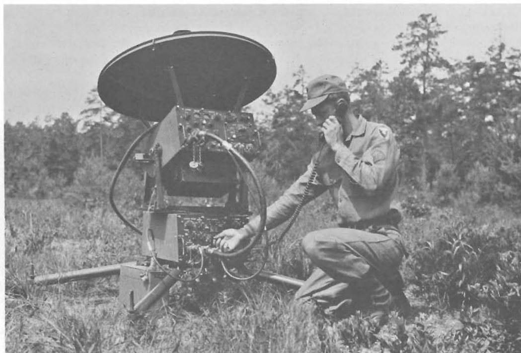
Figure 2. Satellite communications team pack terminal AN/TSC-79.
