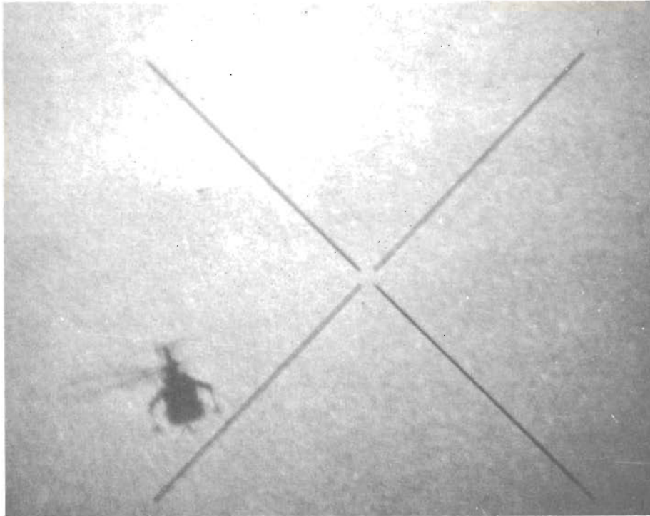
Figure 6. Target helicopter photographed through the night observation device without use of infrared searchlight.
