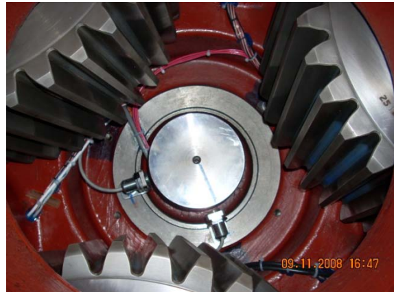
Figure 3. (left) Instrumentation schematic of sun gear for radial measurement, Illustration by Brian McNiff, MLI; (right) installation. NREL PIX 20257
