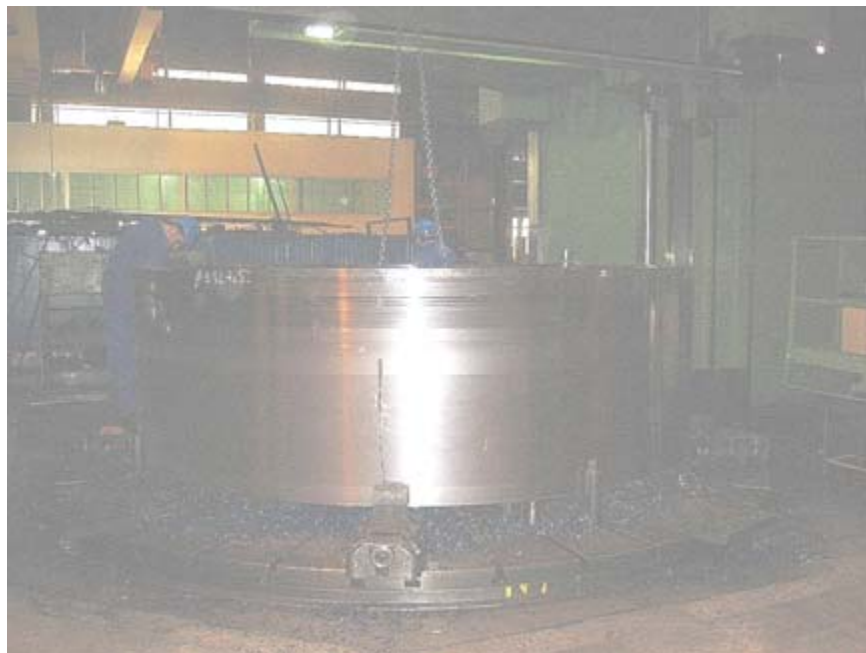
Figure 4-1. The weldment vendor, Felguera, has equipment such as this vertical lathe for machining large parts.
