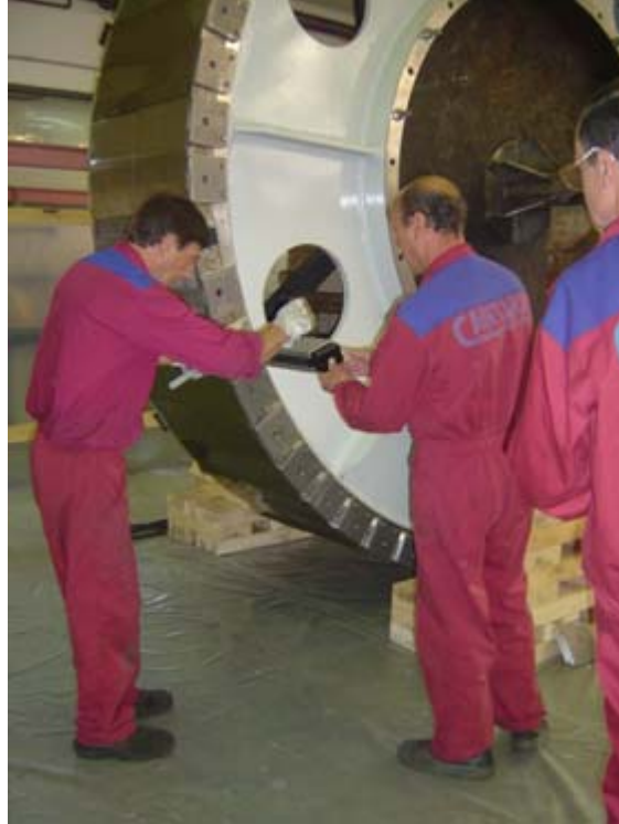
Figure 4-5. The magnets were inserted into the rotor using a proprietary method developed by General Dynamics.
