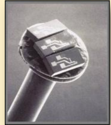
Three MEMS blood pressure sensors on a head of a pin [Photo courtesy of Lucas NovaSensor, Fremont, CA]
