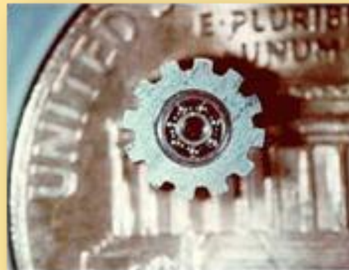
LIGA-micromachined gear for a mini electromagnetic motor [Sandia National Labs]
