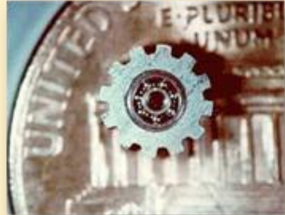
LIGA-micromachined gear for a mini electromagnetic motor [Courtesy of Sandia National Laboratories]
