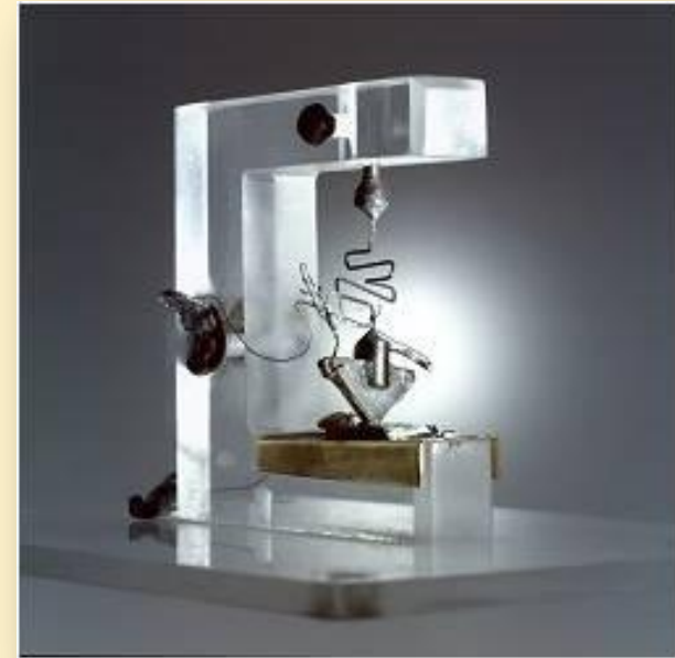
First Point Contact Transistor and Testing Apparatus (1947) [Photo Courtesy of The Porticus Centre]
