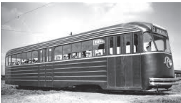
This Pullman Standard 'Model B' was one of the four experimental concepts which evolved into the final PCC streetcar design. Here, the car is on display at Chicago's Navy Pier in August, 1934. Central Electric Railfans Association (CERA)
