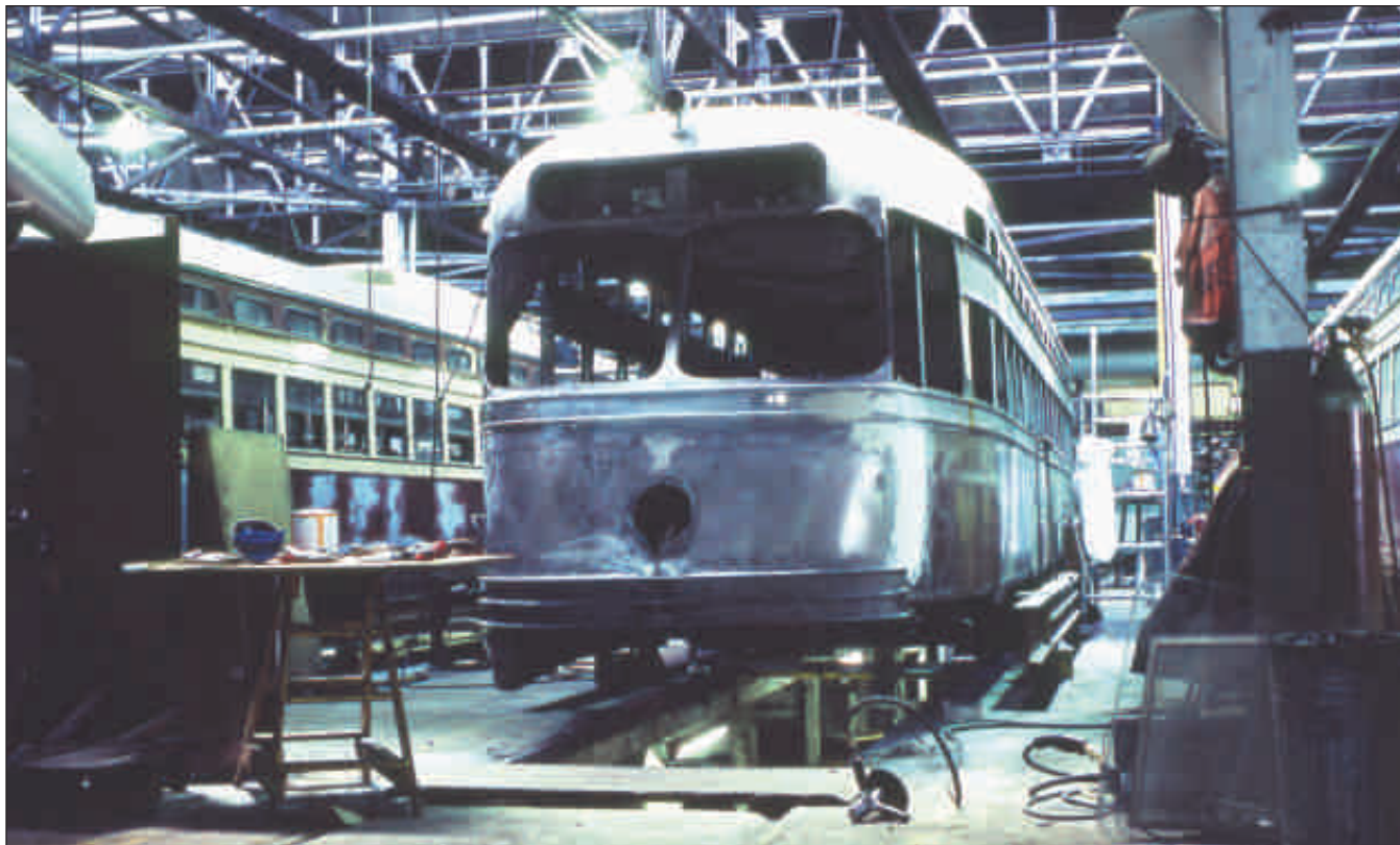
Life extending treatment! The TTC's Hillcrest shops rebuilt 19 PCCs at a cost of $500,000 each in the late 1980s. The cars would be out-shopped as class A15 and renumbered 4600 to 4618. CRHA Archives, Fonds Wickson
