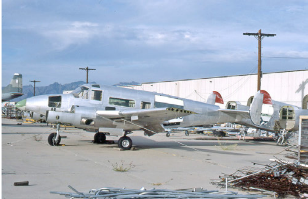
Uncompleted Hamilton Turboliners at Tucson AZ in October 1987 after the conversion line was shut down. Although fitted with E18S style high roof cockpits, these were probably from Hamilton Aircraft Co's stocks of retired military Beech 18 models listed above. Photo by Gordon Reid
