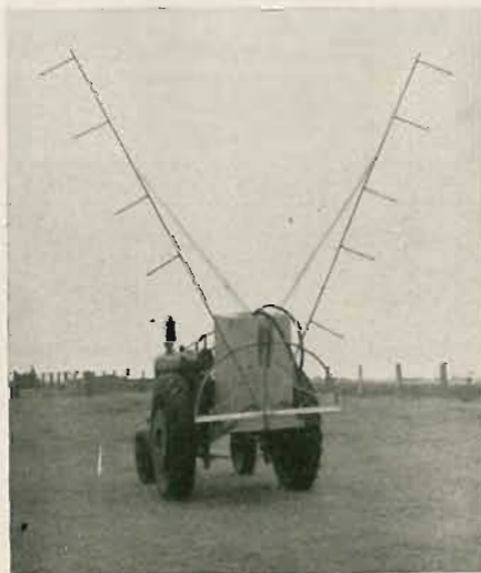
Boom spray on Farmall A.V. tractor. This is used for weed control with 2,4-D.
