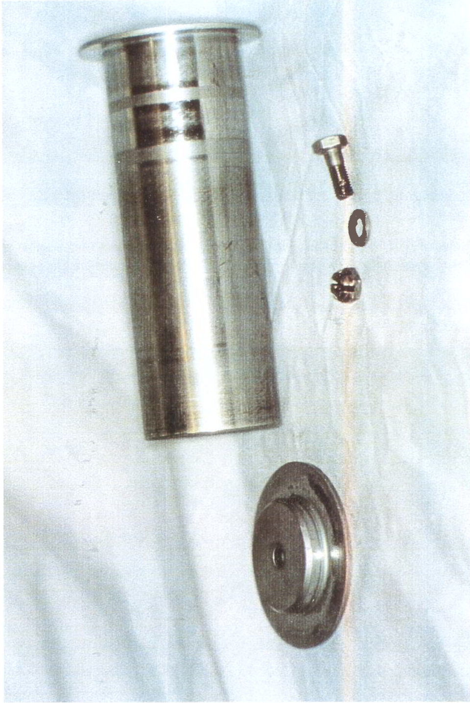
Pin, retainer and fasteners removed from No. 5 position, adjacent to missing parts at No. 6 brake position
