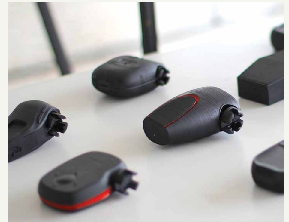
3D printed prototypes for the new Roadie. All prototypes were produced at the Innovation Factory Beirut, a new space for hardware entrepreneurs. (Photo credit: Nadim Choucair)
