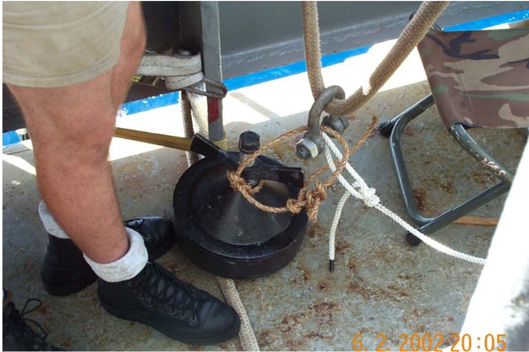
Figure 34. 12" Plug Ready to be Sent Below
