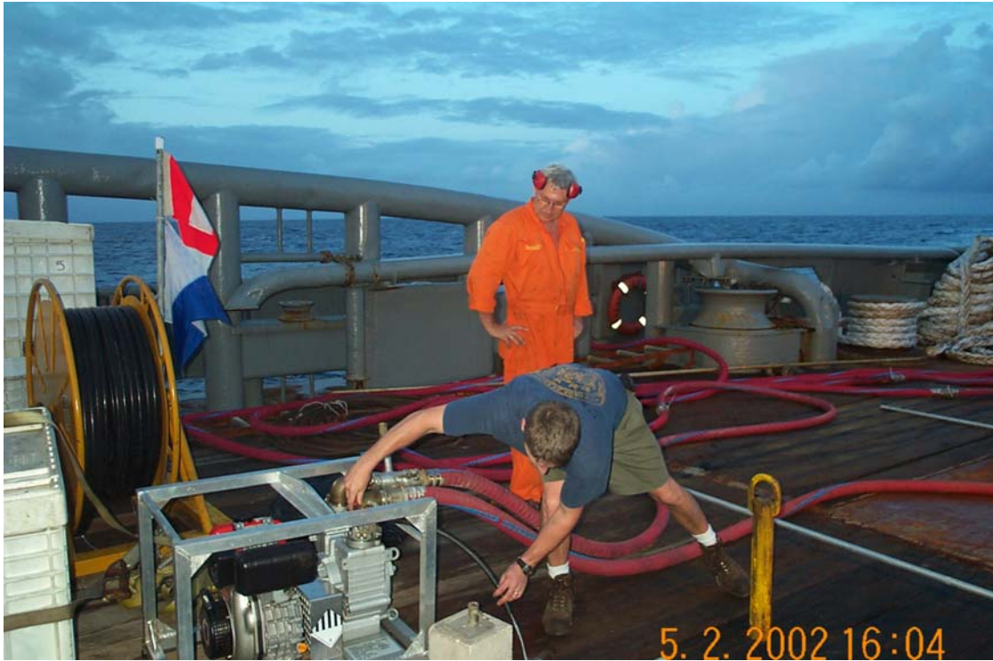
Figure 24. Setting Up Peristaltic Pump
