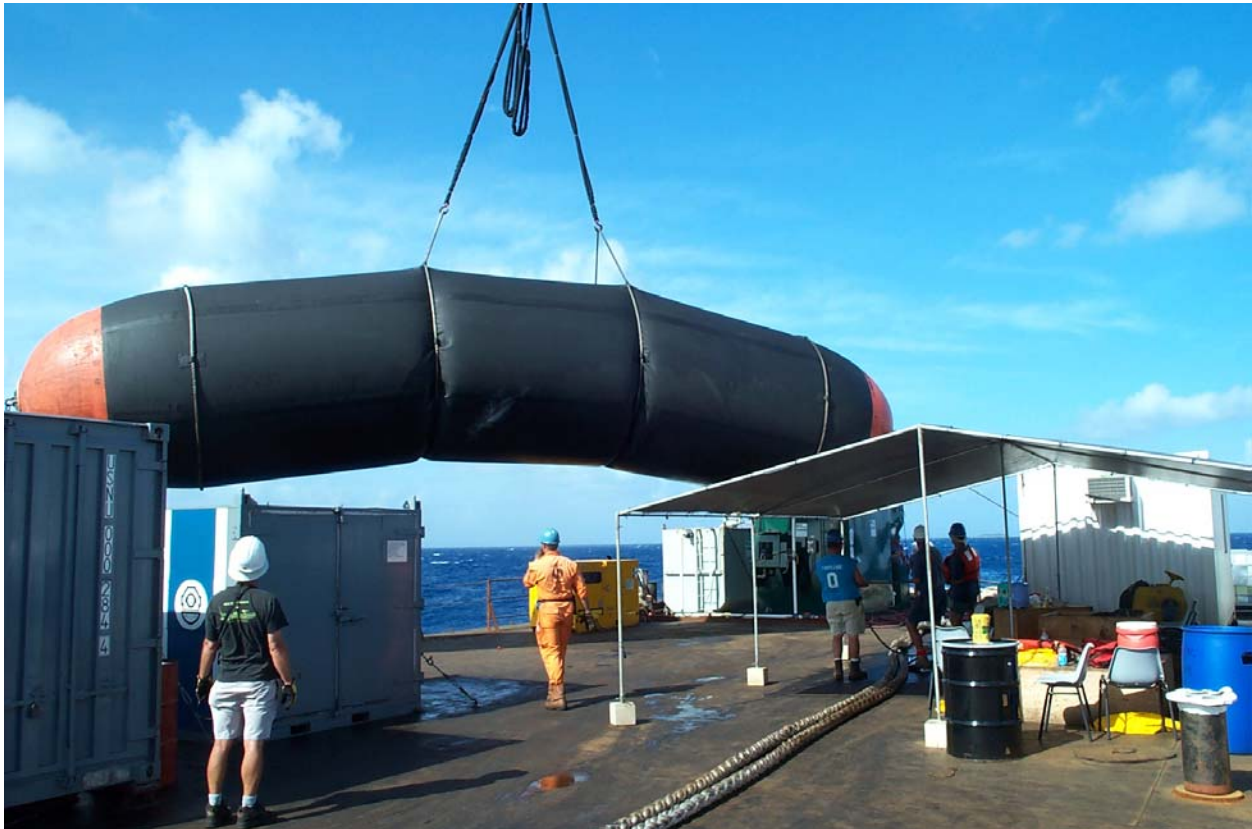
Figure 4-7. One of Four 10' x 50' Fenders Placed Alongside Fels 20
