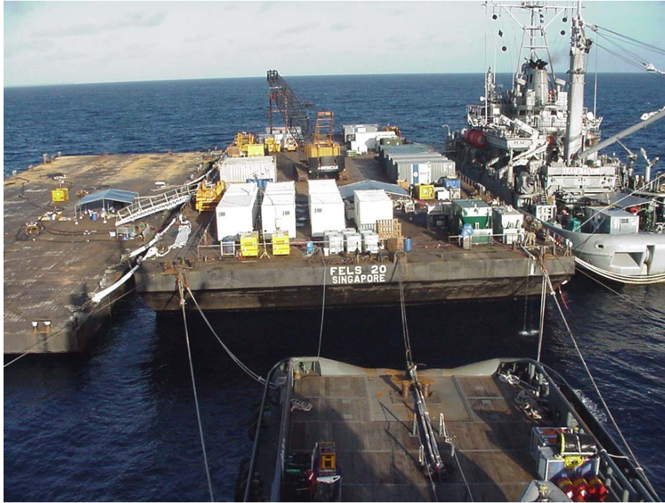
Figure 4-4. Fels 20 Barge In a Six-Point Moor With Fels 21 Barge to Port, Salvor to Starboard, and Seacor Rover to Stern
