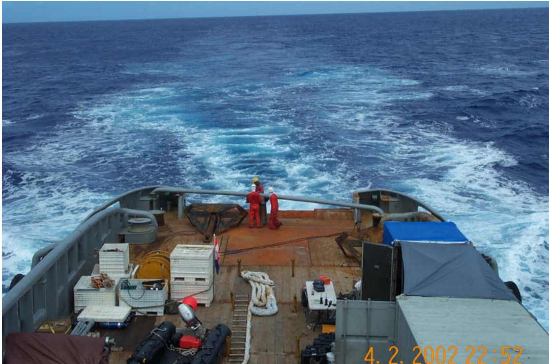
Figure 20. Starboard Stern Anchor Being Prepared for Launching
