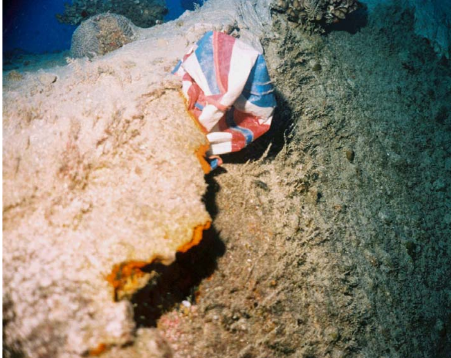
Figure G-3. Hull Crack Patch
