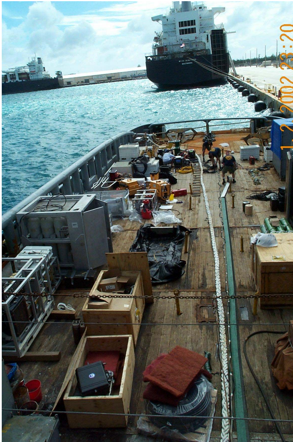
Figure 15. Smit-Lloyd 74 , MDSU and ESSM Equipment Loaded, Stern Mooring Line Down Center of Deck, Anchors, Port and Starboard, Aft
