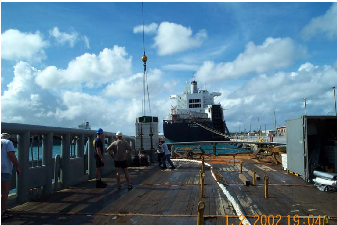
Figure 14. Equipment Loading, Stern Mooring Hawser Down Center of Deck
