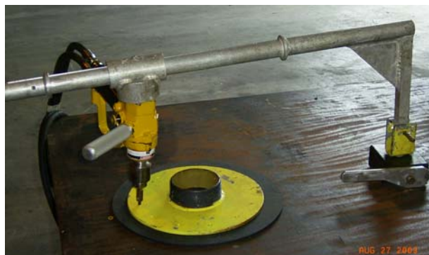
Figure 4-11. "Bubba Bar" and Drill in Position over Flange
