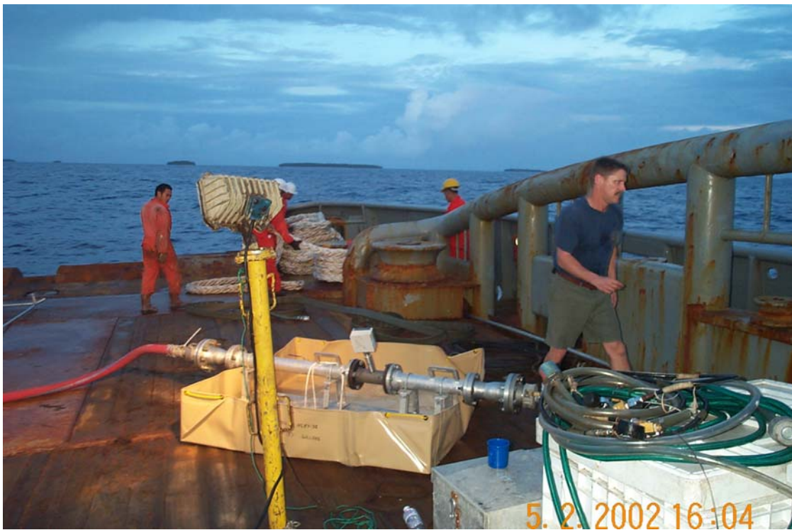
Figure 25. Setting Up Flowmeter
