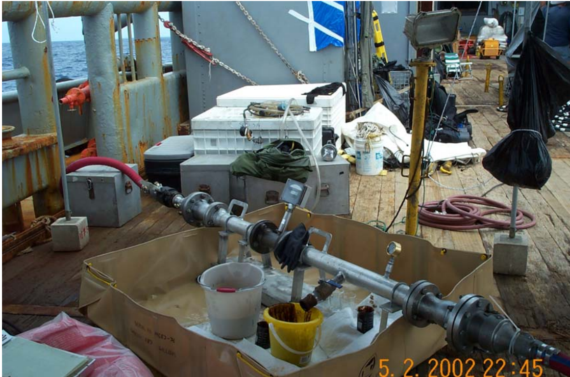
Figure 32. Flow Monitoring and Sampling Station
