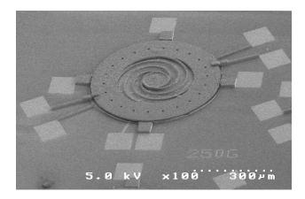
MEMS-fabricated ARL acceleration threshold sensor with spiral springs and individual x/y/z contacts (Image source: ARL)
