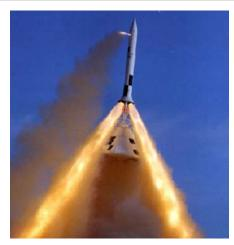
Test flight of Apollo's tower abort system. Image courtesy of NASA
