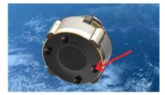
Artist's conception of CST-100 in flight, showing Launch Abort Engines on the aft side of the service module. *Image courtesy of Boeing*
