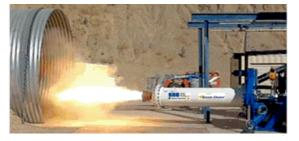
Dream Chaser hybrid motor test firing. Image courtesy of Sierra Nevada
