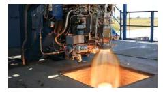
SuperDraco hot fire test. Image courtesy of SpaceX
