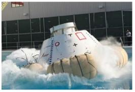
CST-100 water drop test. Image courtesy of Boeing
