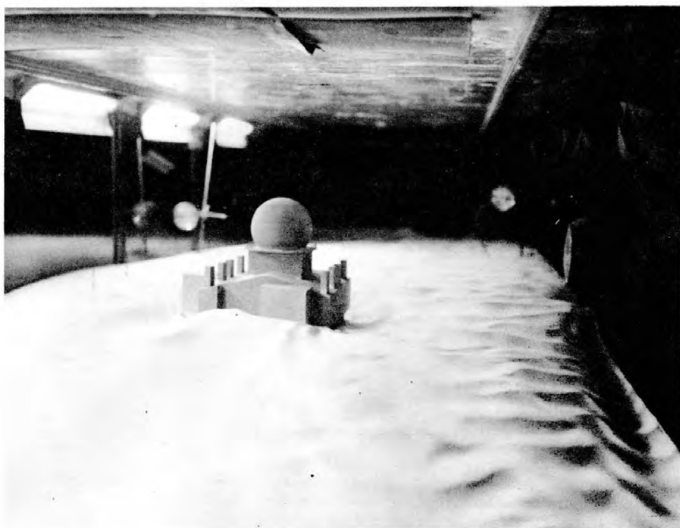
Figure 18. Wind tunnel test of a model of a composite Dye Site building during stages of construction (Gerdel, 1961).
