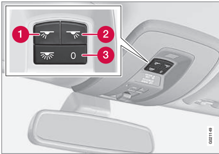
Light switches, front roof lighting
