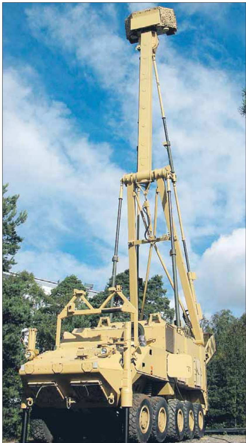
Impressive: The giraffe agile multi beam 740 radar system in extended mode. New counter-rocket and mortar capabilities are bound for Afghanistan.
