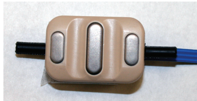
Figure 18-2. Socket electrode used for myoelectric training. This same type of electrode is placed within the myoelectric prosthetic socket. Photograph courtesy of Otto Bock.
