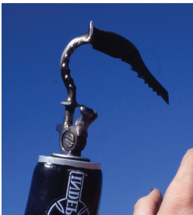
Figure 24-48. Modified split hook for climbing by Pete Davis, accomplished amputee climber. Photograph: Courtesy of TRS Inc, Boulder, Colo.
