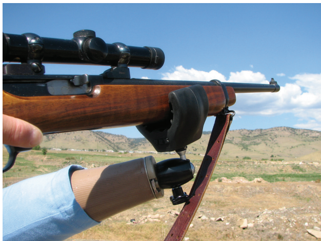
Figure 24-41. Gun turret used with a carbine. Photograph: Courtesy of TRS Inc, Boulder, Colo.
