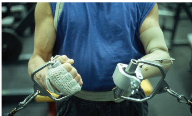
Figure 24-6. Biceps curls with dumbbells using a weight-lifting prosthesis. Photograph: Courtesy of TRS Inc, Boulder, Colo.
