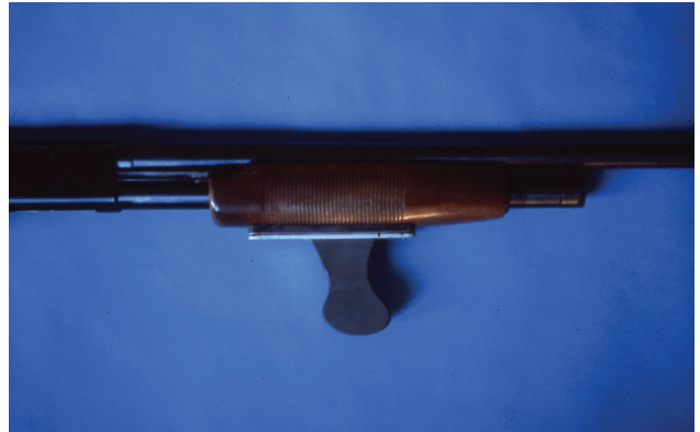
Figure 24-37. Pump style shotgun fore-end modification. Photograph: Courtesy of TRS Inc, Boulder, Colo.
