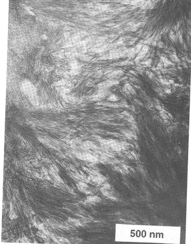
Fine, fibrillar structure, similar to Power's model (typical of Ca/Si > 1.5 )
