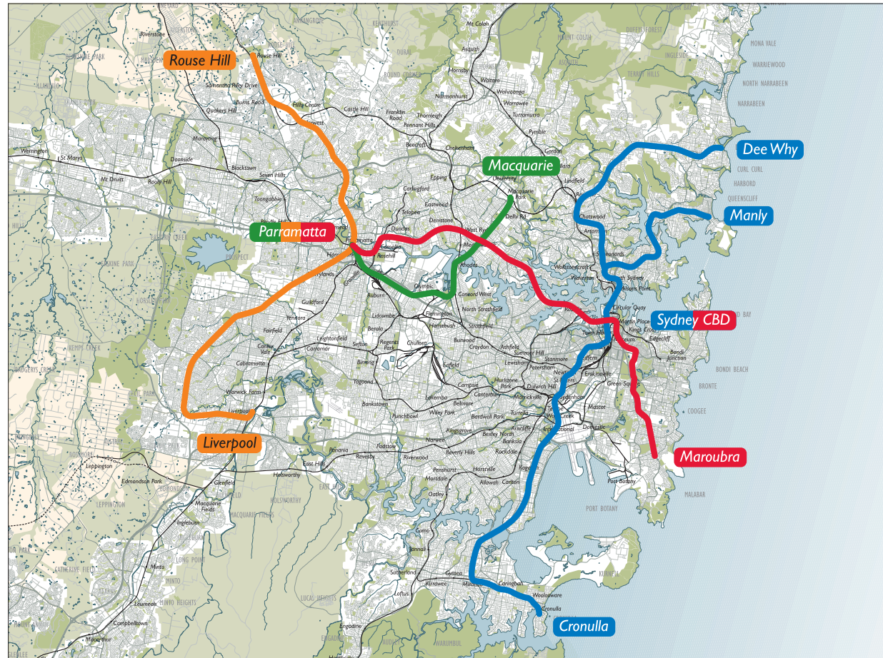
Figure 2. 2005 concepts, based on the 2001 Long-Term Strategic Plan for Rail (“the Christie report”), for additional new lines, operating independently of the CityRail/Sydney Trains network and quite possibly using single deck trains to reduce tunnel construction costs (the savings would be less today) and permit more steeply climbing routes, as the logical next stages of development, but only after MREP or an equivalent had been fully implemented, thereby fully utilising the inherent untapped spare capacity of the CityRail/Sydney Trains system and maximising the benefits of the huge sunk investment in this system.
