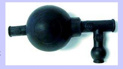
With a gentle twisting motion, insert the pipette into the Safety Pipette Filler about 1/2 cm.
