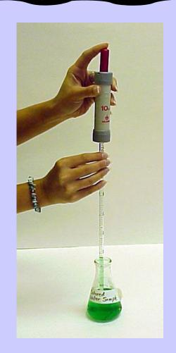
When the pipette is filled to the desired level, touch the tip against the side of the beaker and move the pipette over the waste beaker.
