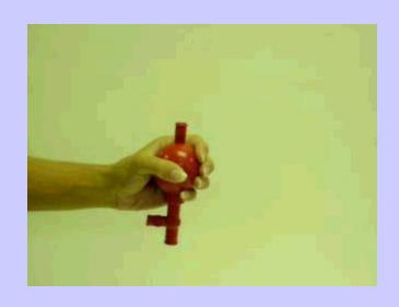
(Click on the picture to see a movie on the SLC computer) To "pull" the liquid up into the pipette place the pipette into the liquid and squeeze the "S" or "suction" valve until the liquid reaches the desired level.
