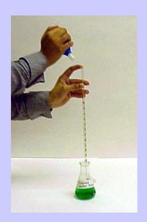
Then raise your finger just enough to allow the bottom of the meniscus to line up with the desired graduation mark. You should observe the meniscus at eye-level while doing this.
