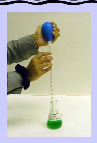
Then quickly, but carefully, remove the bulb as you slip your free index finger over the tip of the mouthpiece hole.
