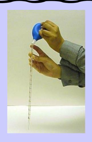
Place the tip into the colored liquid and slowly release the pressure on the bulb.
