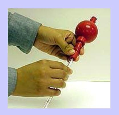
To produce a vacuum for aspiration, squeeze valve "A" with your thumb and index finger of one hand while using your other hand to squeeze the bulb. "A" stands for "air" or "aspirate."
