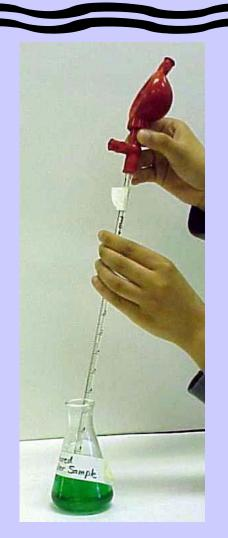
To "expel" the liquid, squeeze the "E" valve. This will allow the liquid to flow out of the pipette except for the last drop.
