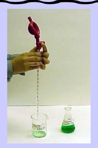
If the last drop of liquid that remains in the tip must be expelled, squeeze valve "E" with your thumb and forefinger, cover the opening in the small bulb with your middle finger and squeeze the small bulb.
