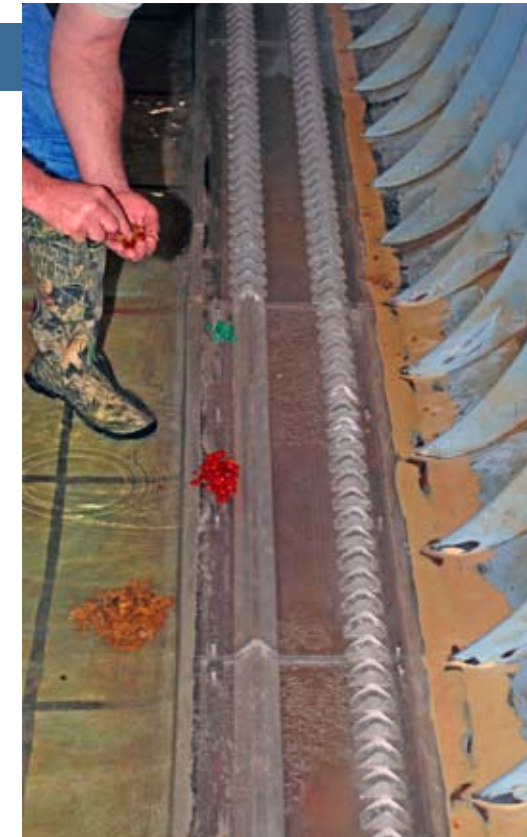
Rocks are placed on the apron of the Bonneville Dam scale model at ERDC. By watching how the rocks move, the team is able to determine how to keep them from jumping onto the stilling basin.
