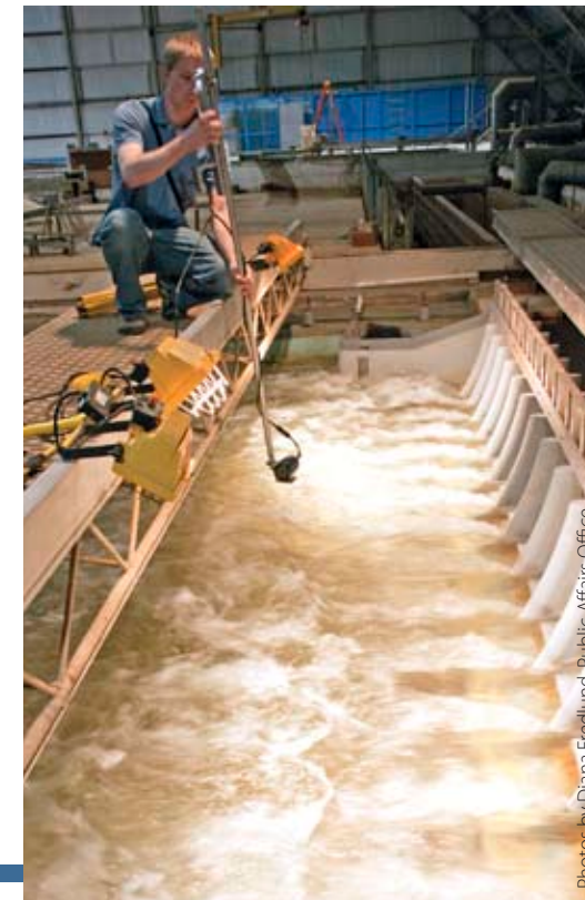
Portland District civil engineer Gary Henrie adjusts the underwater camera to see how the rocks react to different flow levels.
