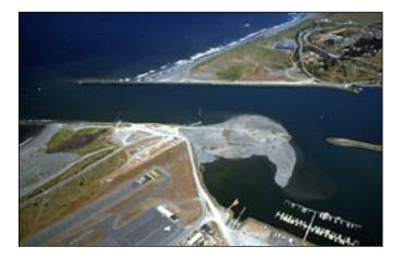
means of alleviating shoaling problems near the river's mouth have been completed. A technical report presenting study findings to date was completed in 1984. The document identified three potential project options: intensive maintenance dredging; jetty extension and maintenance dredging; and a new entrance and maintenance dredging.
