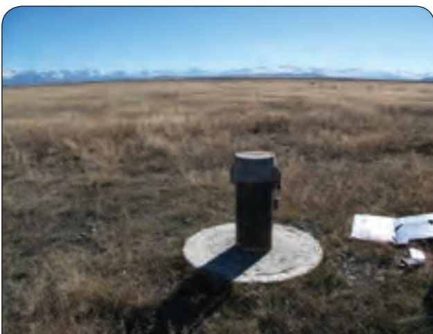
FIGURE 12 // A bore on Gray's Hills Station (adjacent to the Tekapo River) which was assessed for its potential to have a pressure transducer installed.
