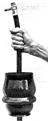
The compactness of the unit, which weighs 9 lb, is demonstrated here. In service, the flexible hose allows for the deflections of the spring and for slight movements of the rubber-mounted sub-frame relative to the hull. Each unit is held firmly in place in its sub-frame by the pre-load on the spring. The damper is well protected
