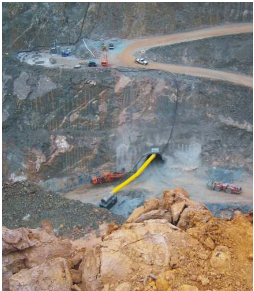
Homestead: portal in Quarters' highwall
