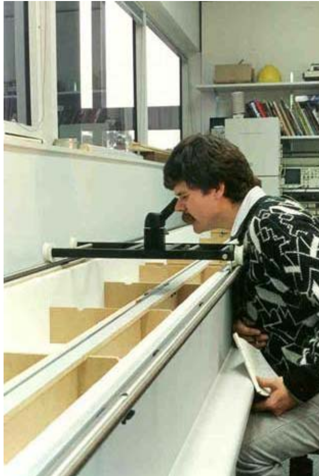
Figure 9 - Calibrating an Aquatrak sensor in a calibration rig.
