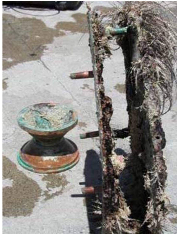
Figure 10 - Biological fouling is a real problem, especially in near shore tropical waters.
