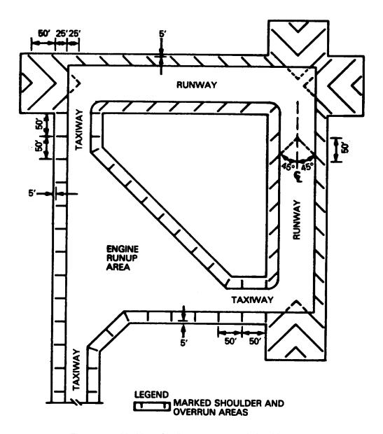
Figure 4-1. Marking of heliport overrun and shoulder area.
