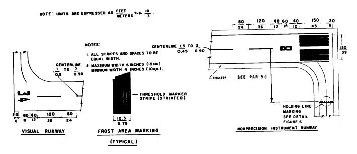
Figure 2-3. Visual and nonprecision marking.
