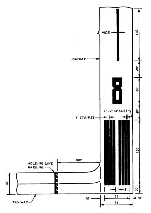
Figure 2-2. Precision instrument runway marking. (Sheet 2 of 2).
