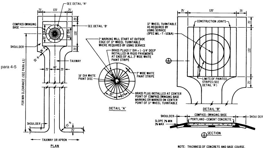
EACH PROPOSED LOCATION FOR A COMPASS-SWINGING ABASE MUST BE CHECKED BY A MAGNETOMETER TO INSURE THAT THE AREA HAS NEGLIGIBLE MAGNETIC CHARACTERISTICS REGARDLESS OF ADHERENCE TO PARA 4-5.
