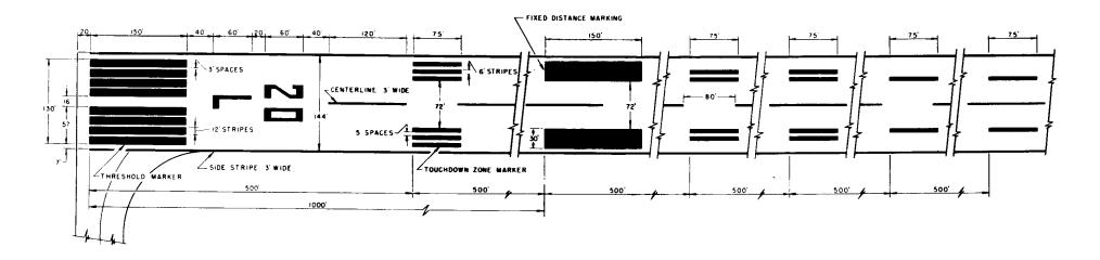
Figure 2-2. Precision instrument runway marking. (Sheet 1 of 2).
