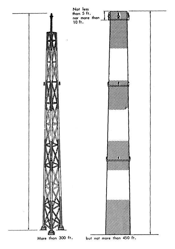
Figure 7-1. Painting and lighting of chimneys, poles, towers and similar obstructions.
