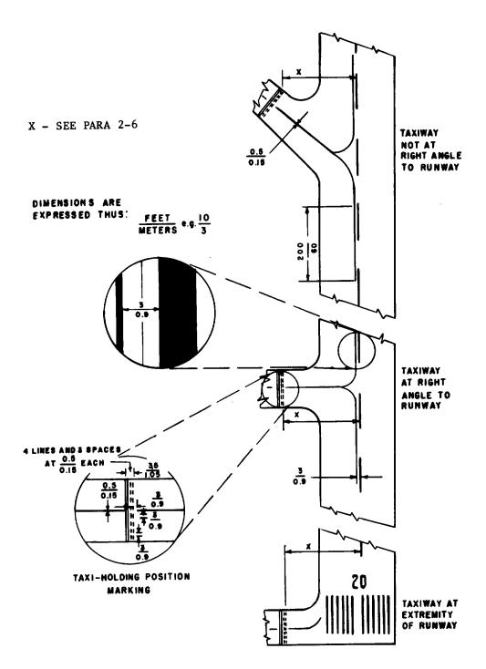
Figure 2-6. Taxiway/runway intersection marking. (Sheet 1 of 2).
