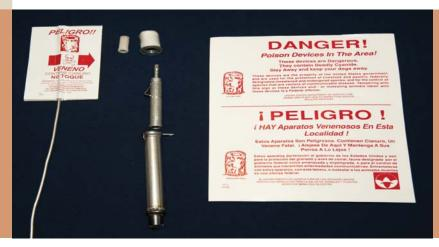
The M-44 device is triggered when a canid (i.e. coyote or wild dog) tugs on the baited capsule holder, releasing the plunger and ejecting sodium cyanide powder into the animal's mouth. The sodium cyanide quickly reacts with moisture in the animal's mouth, releasing hydrogen cyanide gas. Unconsciousness, followed by death, is very quick, normally within 1 to 5 minutes after the device is triggered. Animals killed by sodium cyanide appear to show no overt signs of distress or pain.
