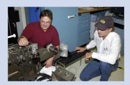
Dr. Chris Immer and Dr. John Lane of Dynacs discuss digital image processing techniques to precisely measure relative positions of the Payload Ground Handling Mechanism (PGHM), which loads cargo into the Orbiter Payload Bay.
