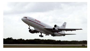
Tucked inside a Pegasus XL rocket, attached to the under belly of the Orbital Stargazer L-1011 aircraft, the HESSI spacecraft lifts off from Cape Canaveral Air Force Station Feb. 5.
