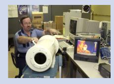
Carl Hallberg of Dynacs demostrates the new Infrared Hydrogen Fire Detection Camera.
