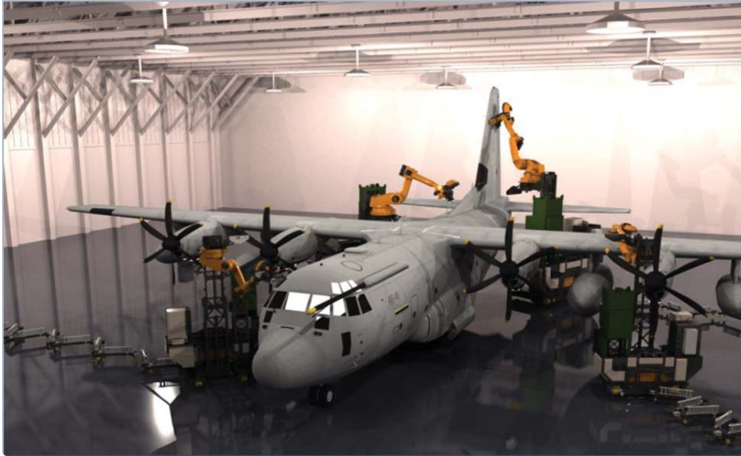
Figure 4 – C-130 Robotic Laser De-Paint Stripping From 2004 Technology Gap to Art of the Possible 2014
