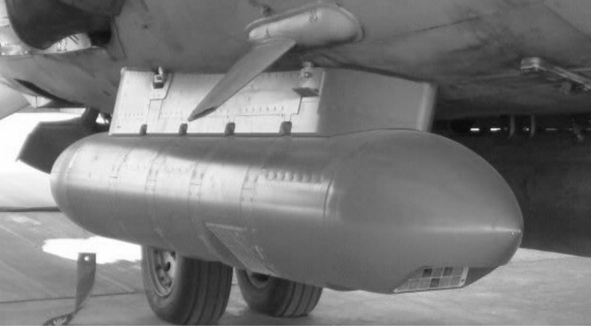
A Terma 1 defensive aids pod; the Terma 2 features the addition of missile approach warning. (MOD)
