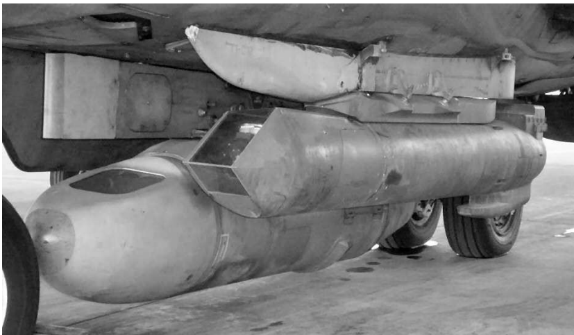
The digital Joint Reconnaissance Pod and (nearest) the Sniper advanced targeting pod on a Harrier's belly hardpoints. (MOD)
