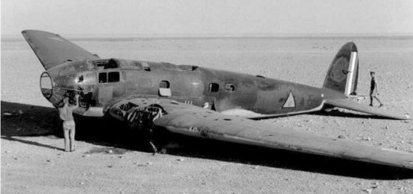
The stripped carcass of a He 111, wearing spurious Iraqi AF markings, that had been forced to land in the desert after being damaged in combat.
