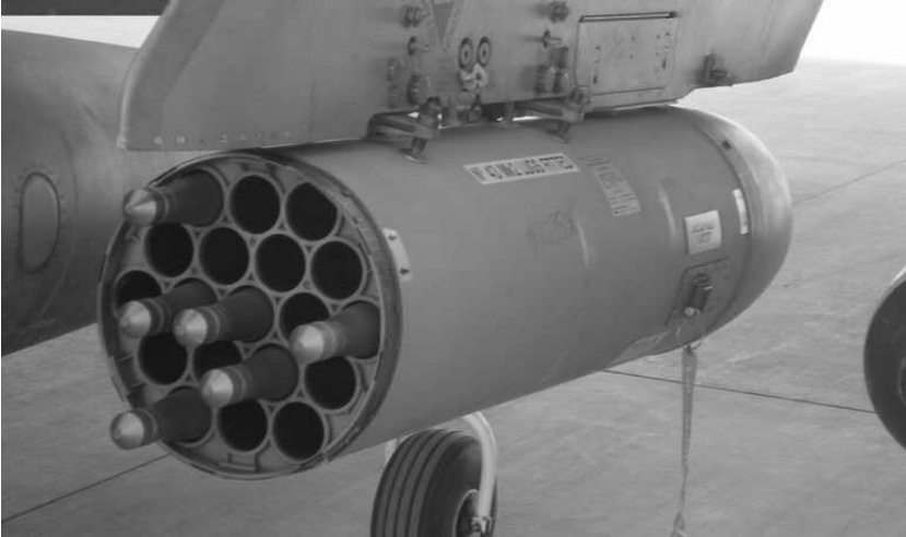
A CRV-7 pod containing nineteen 2.7-inch rocket; until the first rocket is fired, they are protected by a frangible nosecone. (MOD)
