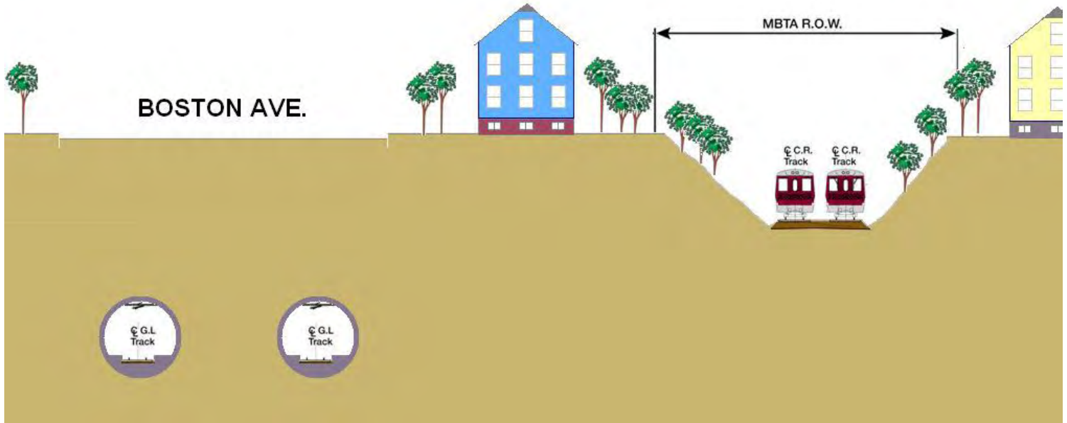
Figure 3-5: Green Line in Deep Bore Tunnel under College Avenue
