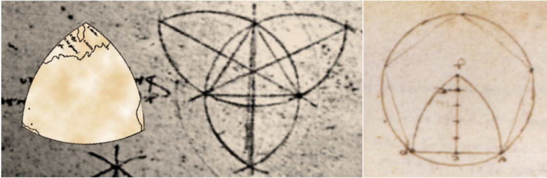
Figure 9. Details of pages from Leonardo da Vinci's notebook developing the geometry of his octant triangle figure, which was later developed as the Reuleaux triangle [12] (Leonardo da Vinci, Paris Manuscript A, 15v; Codex Atlanticus, 923r).
