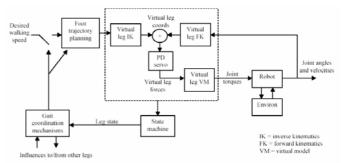
Figure 5: Control Diagram
