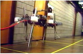
Figure 1. Legged robots developed to study dynamic control and balance. Top: One-legged hopping robot hops in place while responding to a push disturbance delivered by researcher. Bottom: Quadruped robot trots down hallway at about 1.4 m/s (3 mph). Both robotswere powered through hoses by a remote hydraulic pump. These robots were developed in the CMU Leg Laboratory 1981-1986 and the MIT LegLab 1987-1995. To see video of these robots in action, click here: www.BostonDynamics.com/dist/LegLab.wmv
