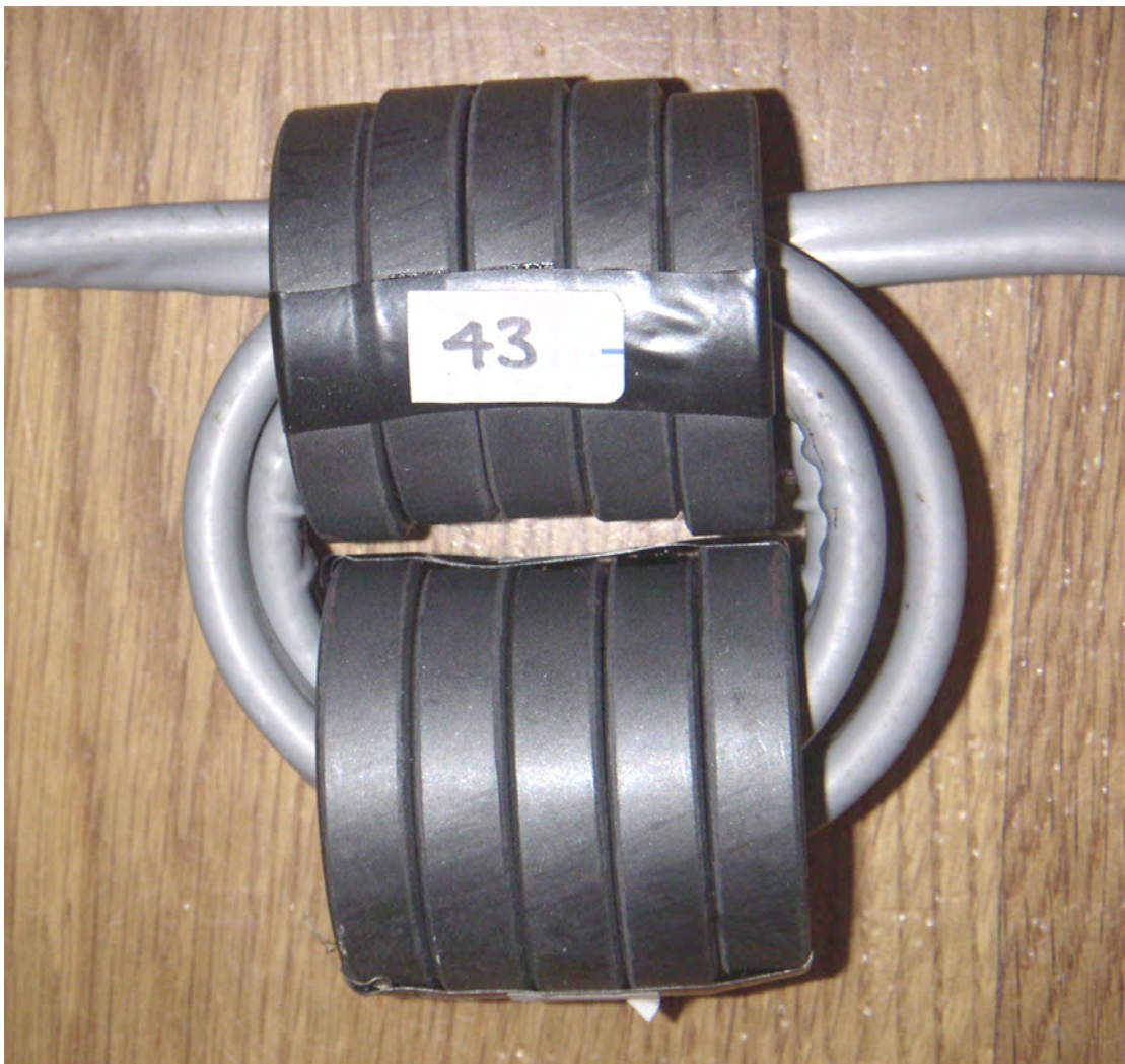
Figure 13: Common-mode choke for a 2 × AWG 4, DC power cable, formed by threading the cable 3½ times through a binocular core formed by two stacks of five Fair-Rite p/n 5943003801, mix-43, “ring” toroids.
