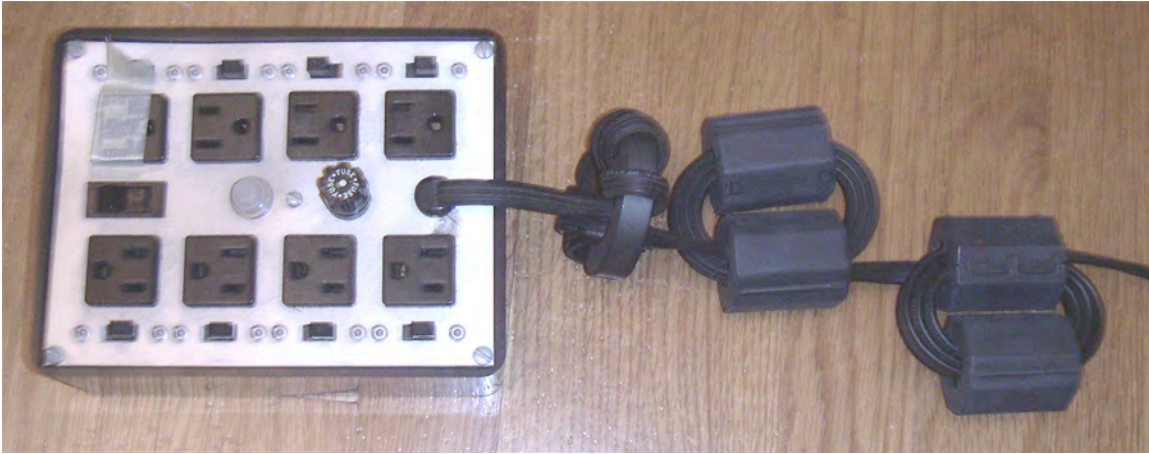
Figure 10: 15-A, 120-VAC, multiple-outlet box including difference-mode EMI filter, fuse, switches, and surge protectors. The toroidal- and two binocular-core ferrite common-mode chokes were added to the line cord.
