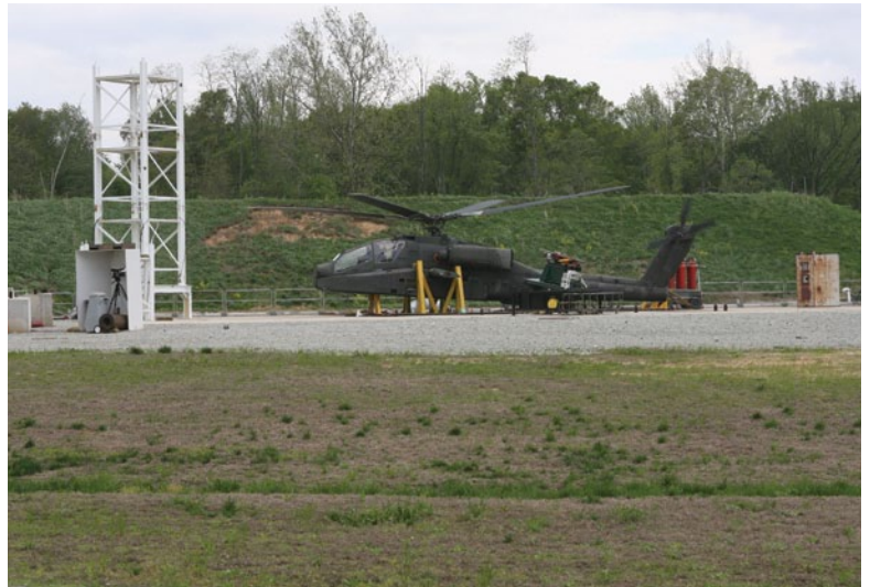
Restrained Apache Block III operating at a flight representative power level on ARL's Rotorcraft Survivability Assessment Facility pad.
