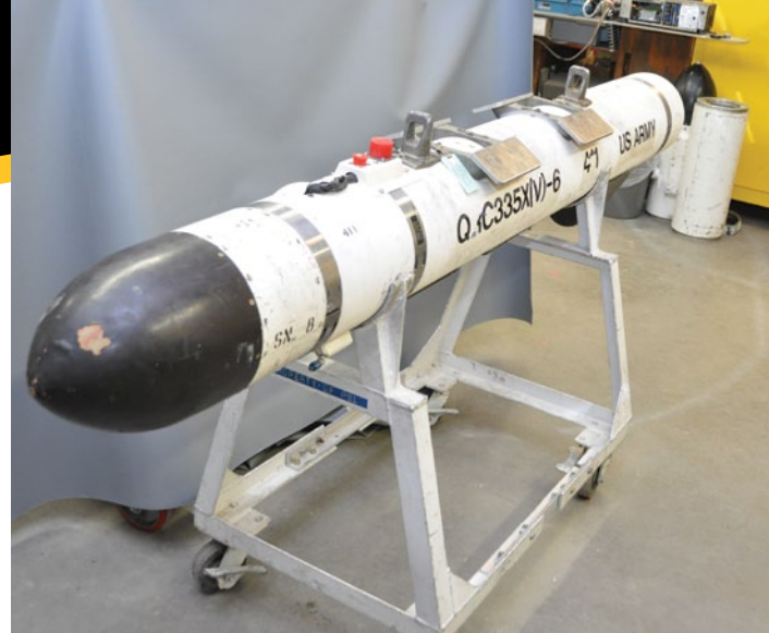
QRC-335 (400) pod is the Army's first DRFM-based airborne EA system in inventory.
