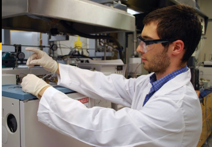
Adam Gamson measuring the biofuel combustion products using gas chromatography analysis.
