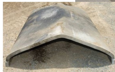
The MAK after the blast test event. The MAK had a permanent deformation of less than 1 inch.
