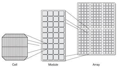
**PHOTOVOLTAIC CELLS, MODULES AND ARRAYS** The building blocks of solar electricity are modular in nature, allowing great flexibility in applications.
