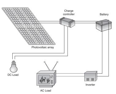
**COMPONENTS OF A TYPICAL OFF-GRID PV SYSTEM** Solar electricity can be used for many purposes, either directly, or by storing in batteries for use when the sun is not shining.
