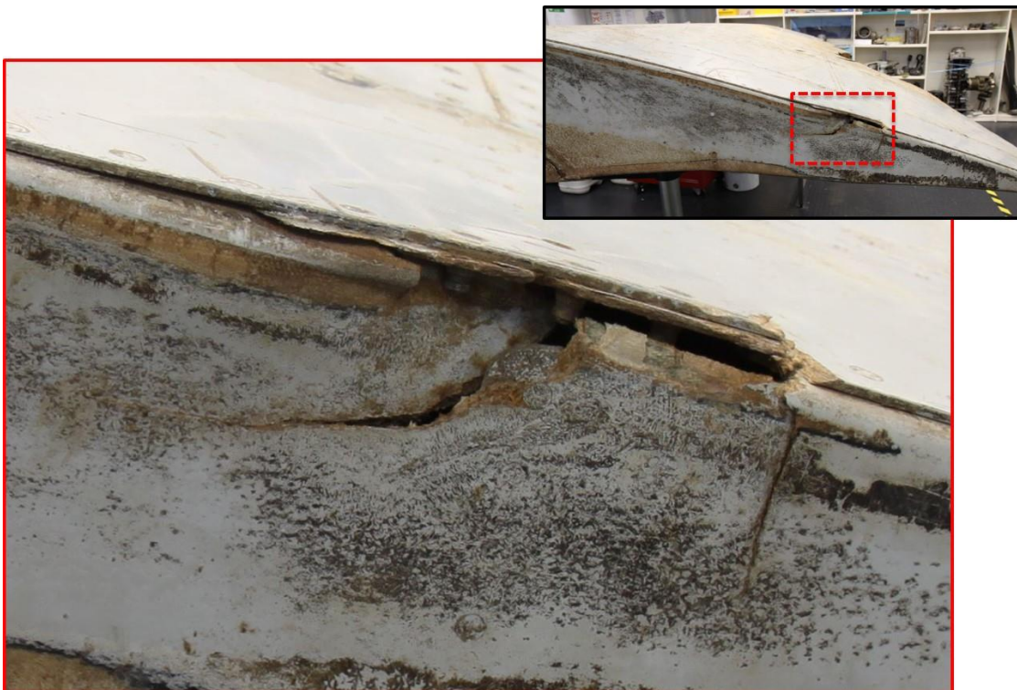
Figure 20: Outboard flap, fractured seal pan (aft)
