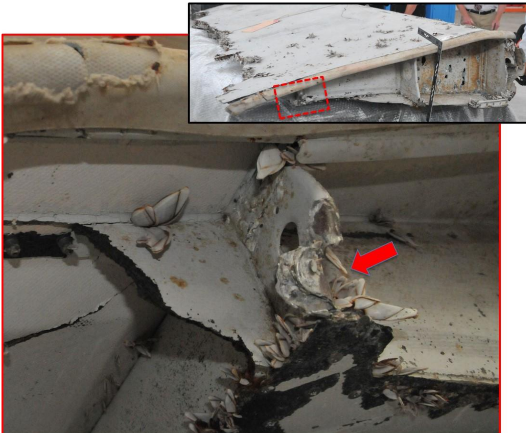
Figure 21: Flaperon, outboard side damage
