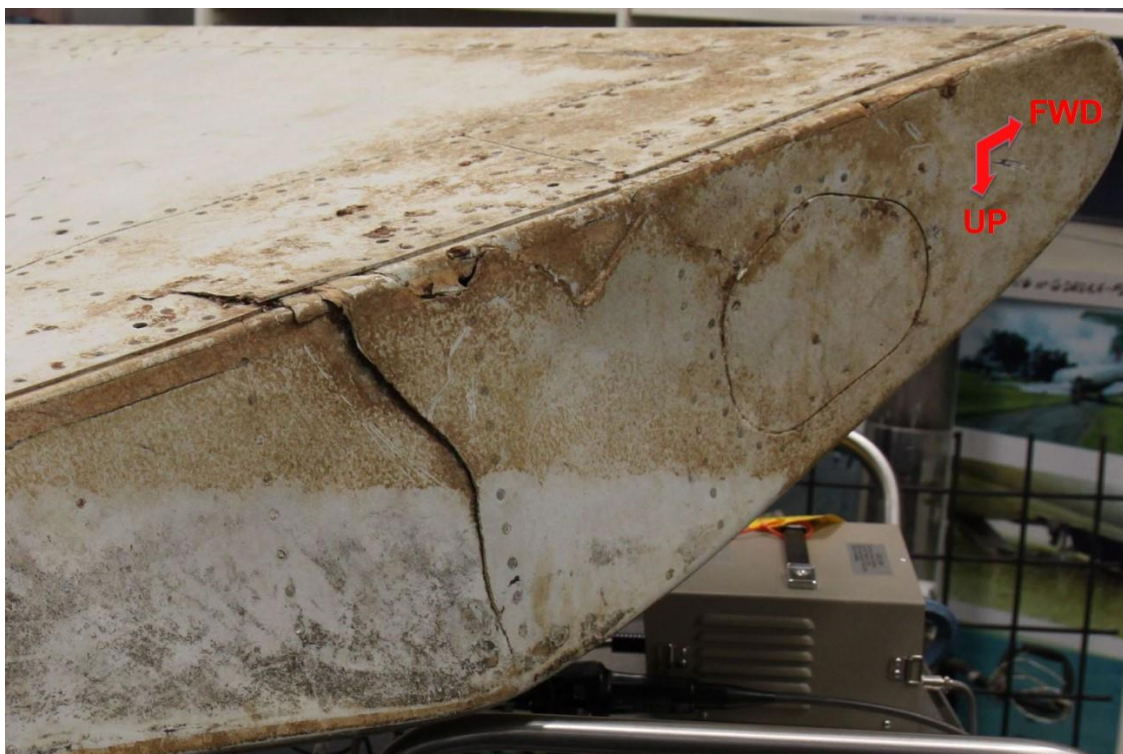
Figure 19: Outboard flap, fractured seal pan (forward)
