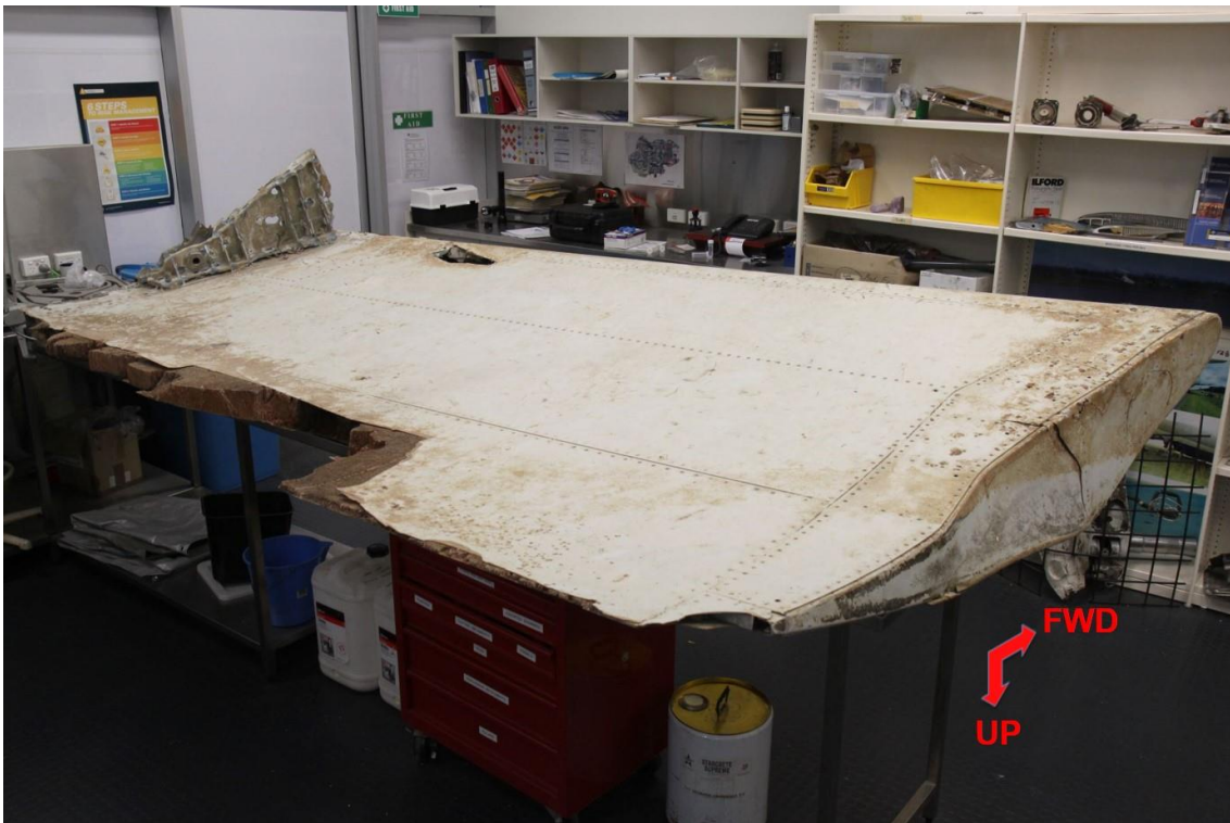
Figure 14: Inboard section of outboard flap (inverted)
