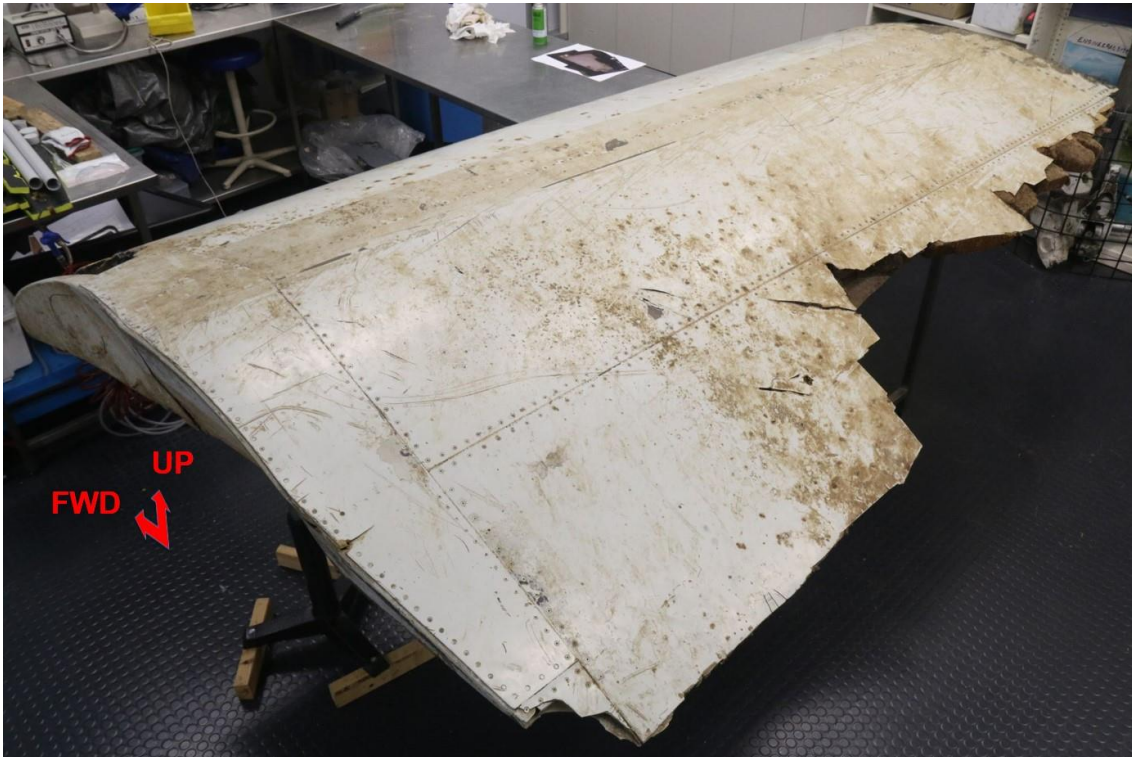
Figure 13: Inboard section of outboard flap
